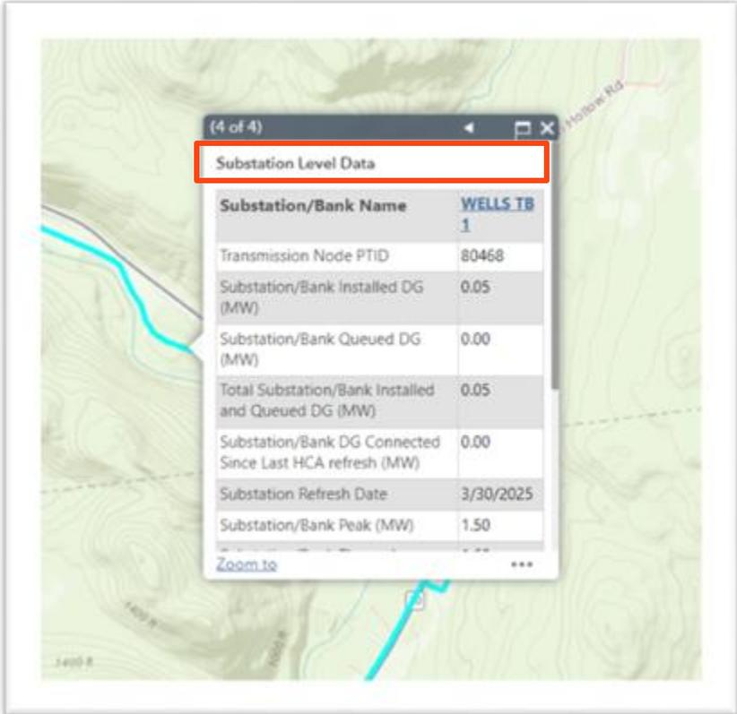
The screenshot shows a topographic map with a cyan line representing a substation. A pop-up window titled "Substation Level Data" is overlaid on the map. The window contains a table with the following data:
